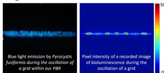
For our experiments, we considered the PBR in the same configuration as for the PIV experiments with a simple cartesian grid,  $A = 50$  mm and  $\nu = 0.5$  Hz. The bioluminescence images were recorded with a CMOS camera LaVision Imager M-lite 5M.
